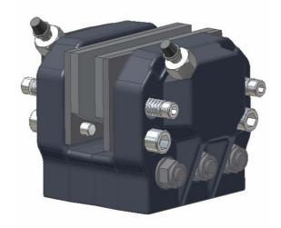
Two springs on each brake half retract the brake pads from the disc when pressure is released. Brake pad wear is automatically compensated for with increased piston stroke.
