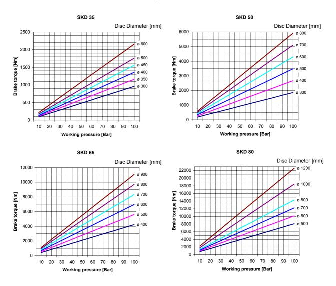
The braking torque is calculated from the following formula:
