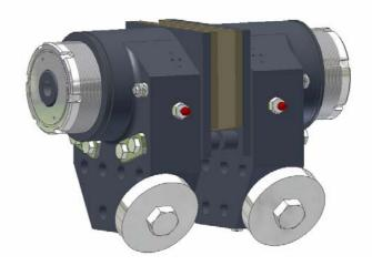
Each brake half has two cylindrical guide pins that transmit the tangential braking force from the brake lining to the brake housing and support. As a result, any radial forces on the brake pistons are minimized which contributes to longer brake life.
