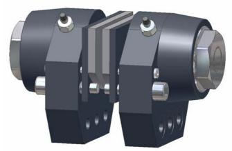
Each brake half has two cylindrical guide pins that transmit the tangential braking force from the brake lining to the brake housing and support. As a result, any radial forces on the brake pistons are minimized which contributes to longer brake life.
